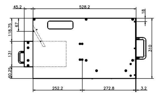
The crate has 19" width and 7U height dimensions. The maximum deep of module is 625mm. Module enclosure corresponds to standard DOE/ER-0457T.
