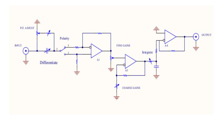
Fig. 1. Block Diagram of the NCB226 Fast-Filter Amplifier.
